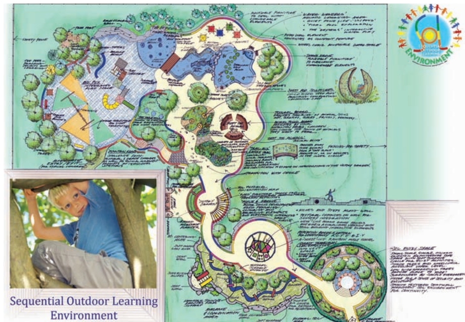
Tara Vincenta has developed guidelines for consideration when designing outdoor environments for children with ASDs. This is a plan view of an outdoor environment designed using these guidelines; however, many of these guidelines can be creatively integrated into existing outdoor play spaces.
