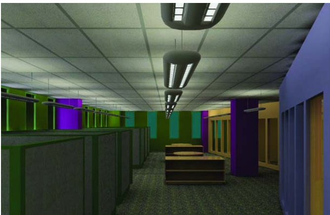
GSA Study: Indirect/Direct Lighting
