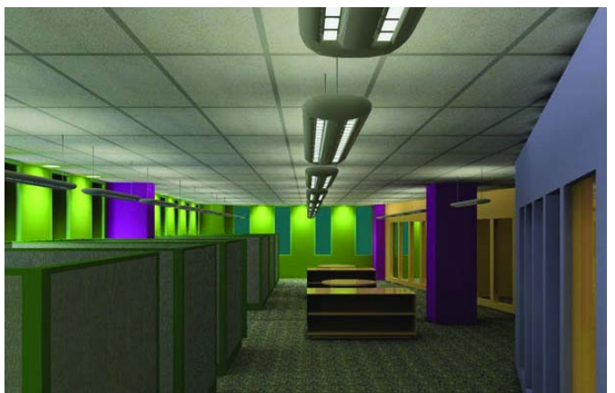
GSA Study: Indirect/Direct Lighting with Wall Wash
