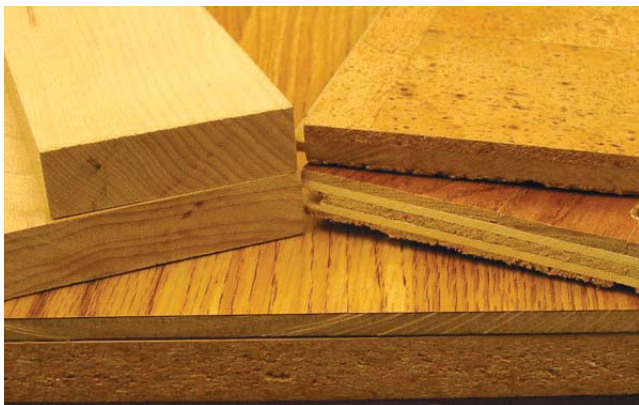
Which wood should be selected? Laminated with a particle board base, pre-finished with a plywood base, solid wood finished on site or cork?
